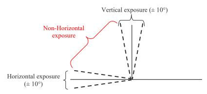
• The real durability of a product depends on a large number of parameters, including, among others, the quality and preparation of the substrate, exposure (environment, climate, exposure angle), graphics maintenance, and degree of pollution.
