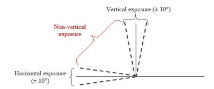
• The real durability of a product depends on a large number of parameters, including, among others, the quality and preparation of the substrate, exposure (environment, climate, exposure angle), graphics maintenance, and degree of pollution.
