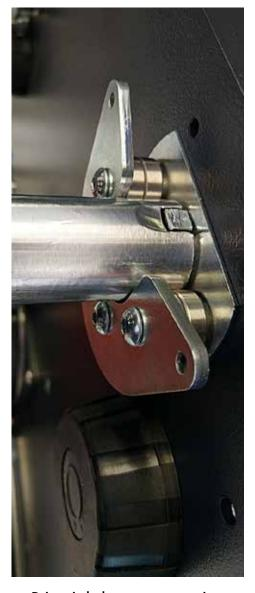
Drive via bolt-groove connection
