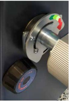
Brakes and slip clutches for all axles
